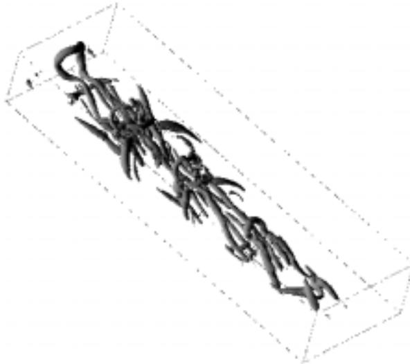
FIGURE 5. Iso-surface of the imaginary part of the eigenvalue of deformation rate tensor. The figure show the eigenvalue calculated from the same velocity field as in figure 4. Contour level at 0.32.
